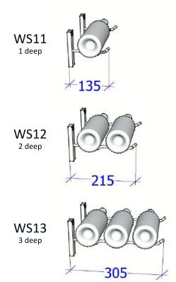
Standard column width is 330mm (can be reduced by interleaving)
